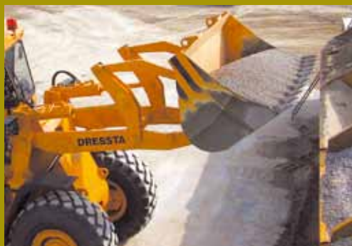
Rock bucket, with teeth, for use with tool carrier
