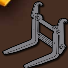
Fork-lift attachment for use with tool carrier
