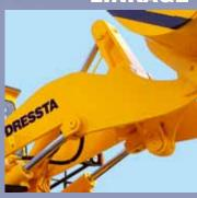
Z-Bar linkage transfers maximu force to the bucket to pry out hamaterial.
