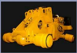
The front frame with high mount boom cylinder pivots increased lifting ability to the top without sacrificing digging ability. The rear frame features trunion rear axle mountings.
